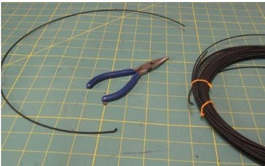
Black millinery wire, #18 gauge. By using black wire with black fabric I didn't have to cover the wire with ribbon or fabric. You will see the wire because the fabric is sheer.
